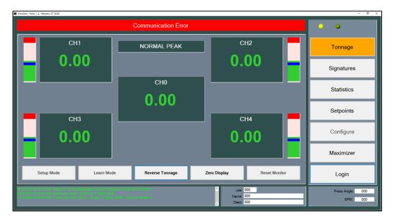
When you first start SlimWare, you will notice that the communication lights in the top right-hand corner are not flashing, and you get the following message in the status window at the bottom. This indicates that communication is not yet established.
