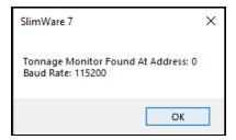
If the search ends with no device found, check the communication cable, and verify that the correct com port is selected in SlimWare.
