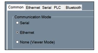
On the Common tab, verify that the communication mode is set to Ethernet. If not, select it.
