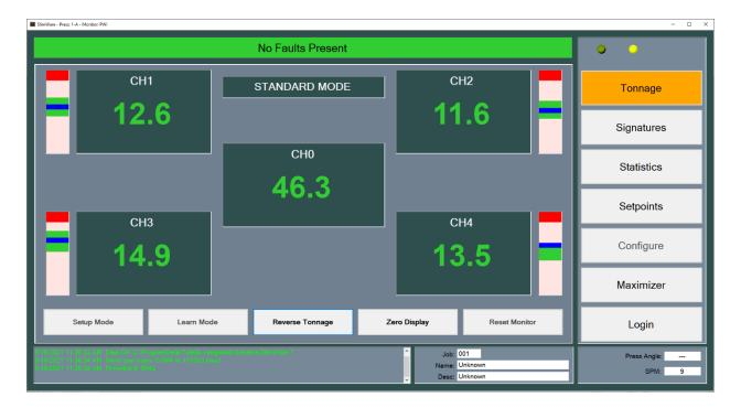
Figure 5-1 – Tonnage Screen (4 Channel)
