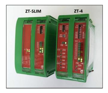
For the ZT-Series tonnage monitor to display accurate tonnage information, the unit must be properly calibrated. Calibration is performed by using SlimWare and the ZT-4 module (see above).
