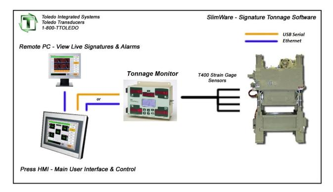
Figure 1.1 – Tonnage Monitor / SlimWare System Overview
