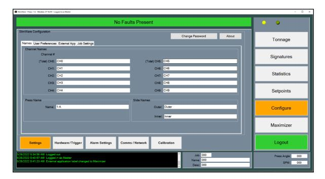
Figure 9-1 - Configuration Settings Screen
