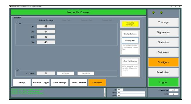
c) Push the "Display Balance/Gain" button. The gain values are shown in the "Balance/Gain" column.
