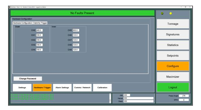
Figure 9-6 - Capacity Screen
