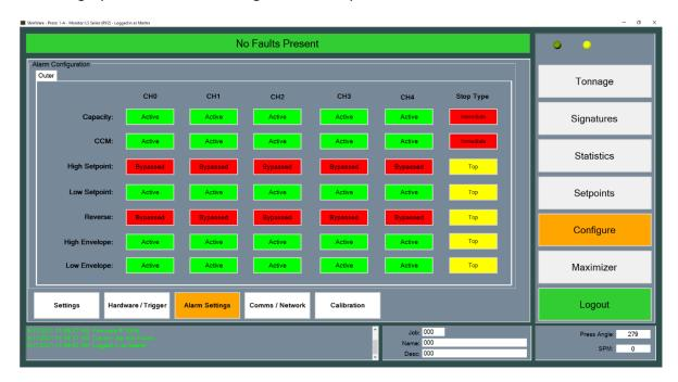
Figure 9-8 Configuration Bypass Screen (4 Channel)
