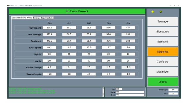
Figure 8-1 – Setpoints Screen (4 Channel)
