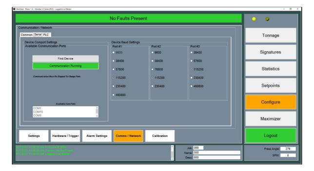
Figure 9-11 Configuration Communication/Network Serial Screen
