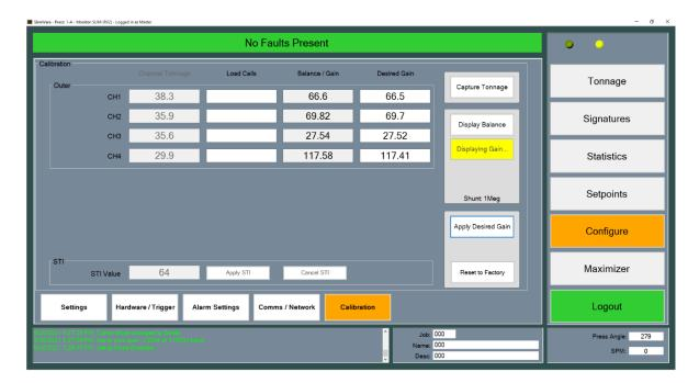
i) Push the "Capture Tonnage" button and cycle the press. The values in the "Channel Tonnage" column should match the load cells. If not, repeat from Step 7d.
