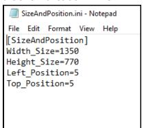
Width\_Size is the width of the SlimWare window, in pixels. Height\_Size is the height of the SlimWare window, in pixels. Left\_Position is the distance in pixels from the left edge of the screen.
