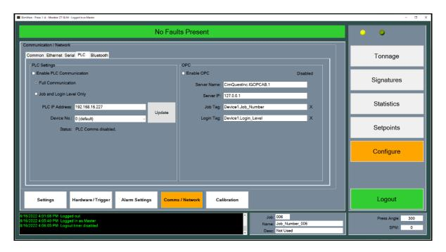
Figure 9-12 Configuration Communication/Network PLC Screen
