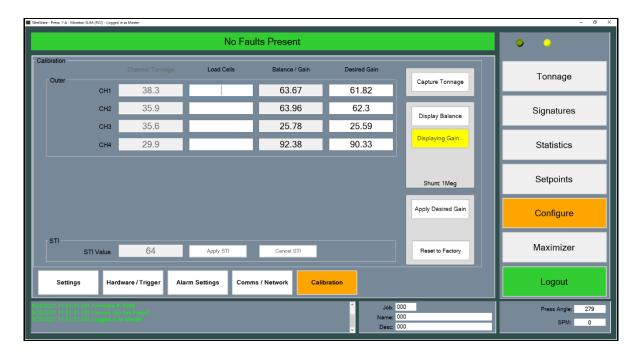
Figure 9-15 Configuration Tonnage Calibration Screen (4 Channel) – SLIM/LS-Series
