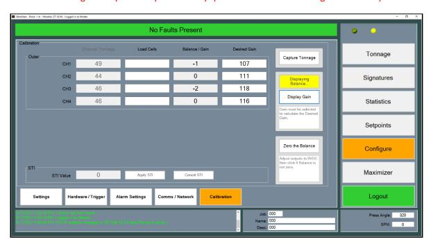
Figure 9-14 Configuration Tonnage Calibration Screen (4 Channel) – ZT-Series Monitor
