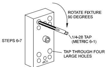
STEP 6 Loosen the fixture. Rotate the fixture another 90 degrees clockwise such that the larger corner holes line up with the holes drilled in Step 4. Insert a tap to be sure the holes line up. Lock the fixture in place by tightening the center screw.
