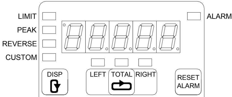
The N600 has four data types that can be displayed on the screen. To select the display press
