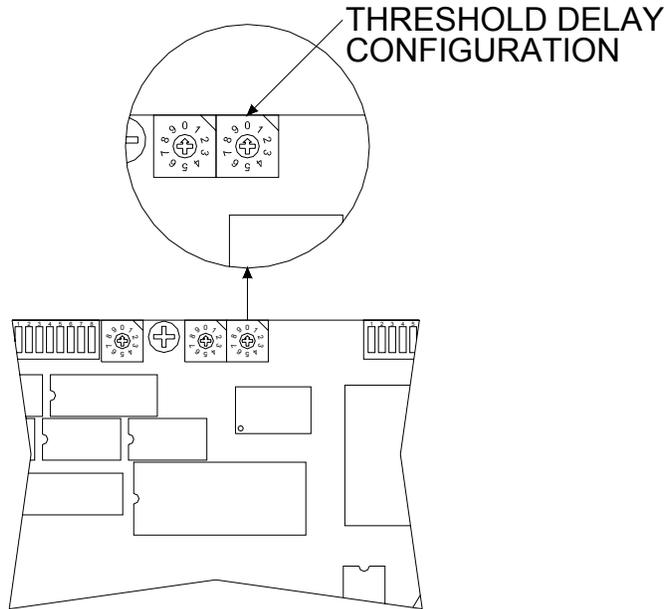
**Figure 2.5: Threshold Delay Configuration**
