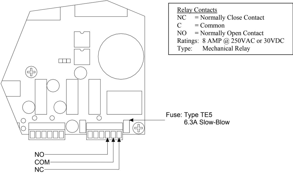
**Figure 1.19: Shutdown Relay Wiring**
