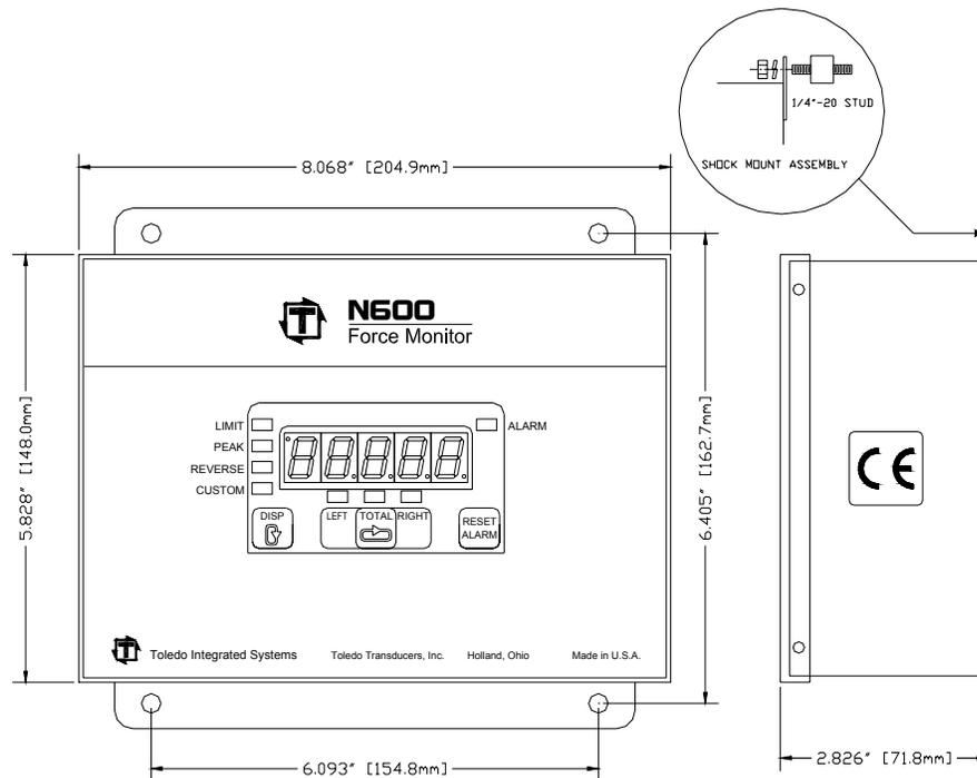
**Figure 1.1: Standard Mounting Dimensions**
