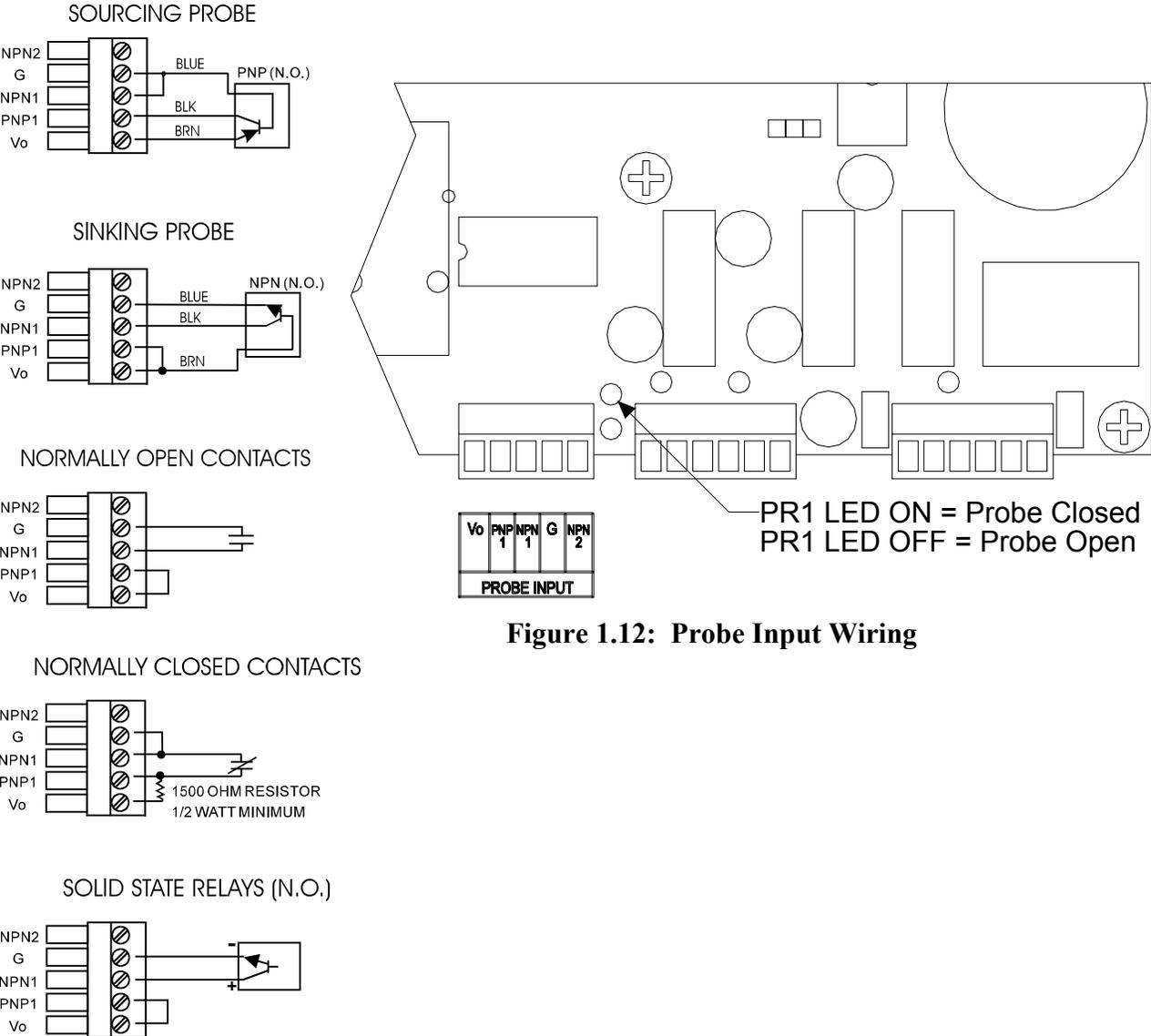
Figure 1.12: Probe Input Wiring
