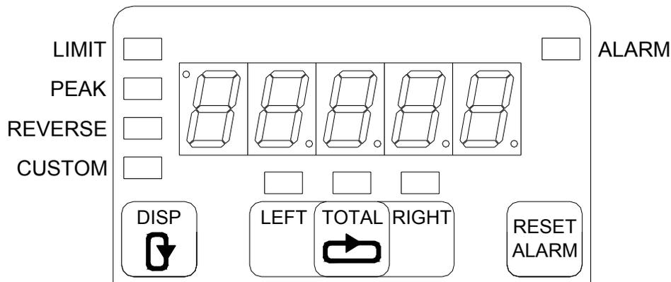
The layout of the 7-segment LED display and the eight other LED's are designed to be simple and require little explanation.
