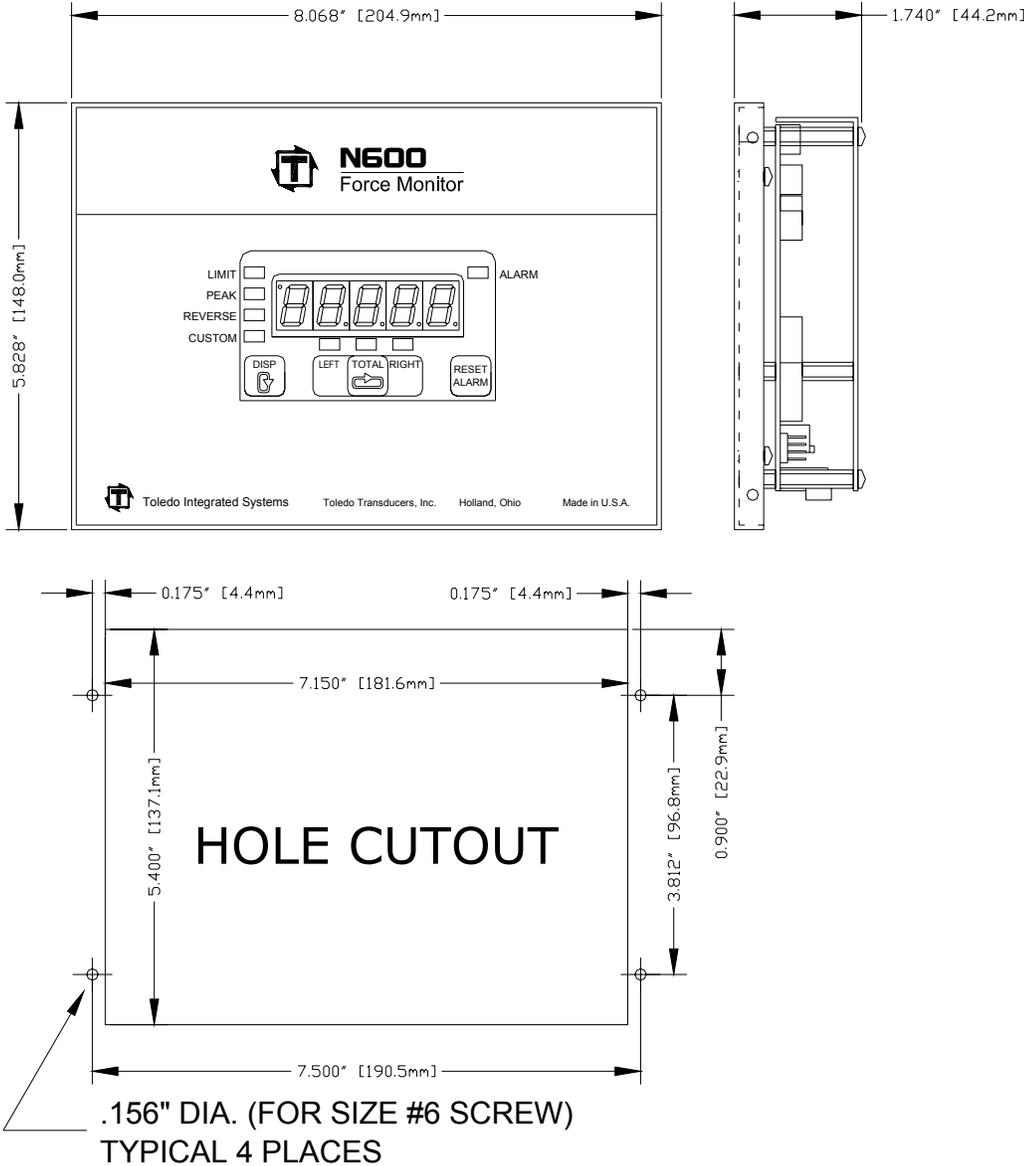
**Figure 1.2: Flush Mount Mounting Dimensions**
