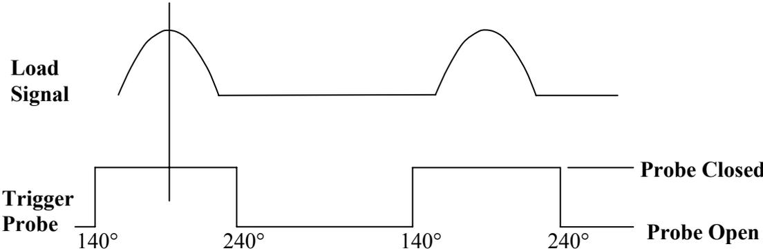
Figure 1.13: Probe Timing
