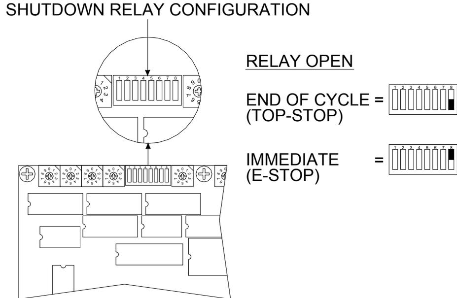
**Figure 2.9: Shutdown Configuration**
