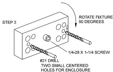
STEP 3 Bolt the fixture to the press member using the 1/4-28 by 1-1/4 inch long socket head cap screw in the center of the fixture. Orient the fixture as shown and drill out the #21 holes to a depth of 3/8 of an inch for the enclosure mounting. The fixture is not used for tapping these holes. (Optional)
