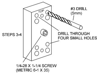
STEP 3 Bolt the fixture to the press member using the ¼-28 by 1-¼ inch (M6-1 x 35) long socket head cap screw in the center of the fixture.
