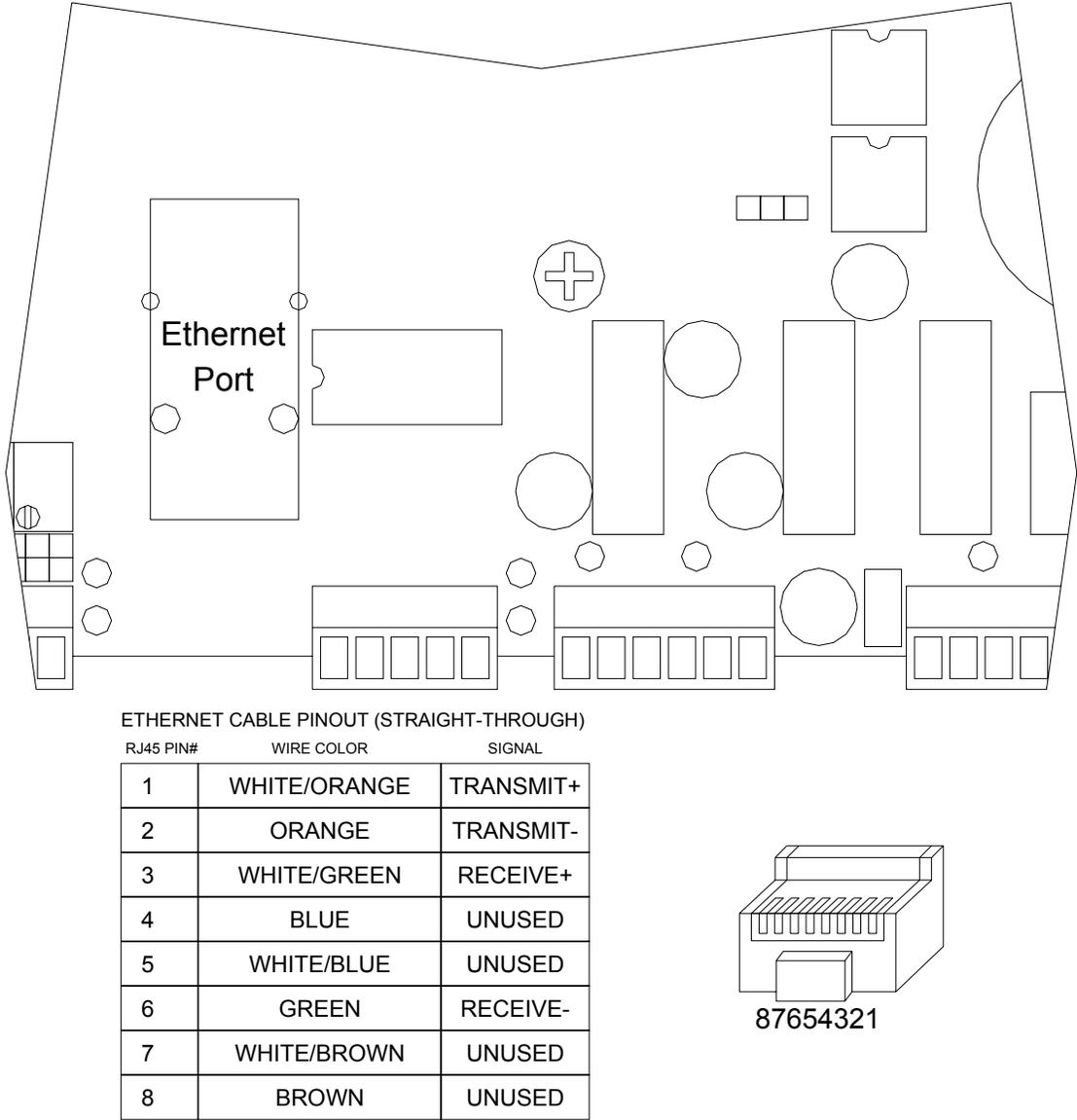
Figure 1.18: Ethernet Connection
