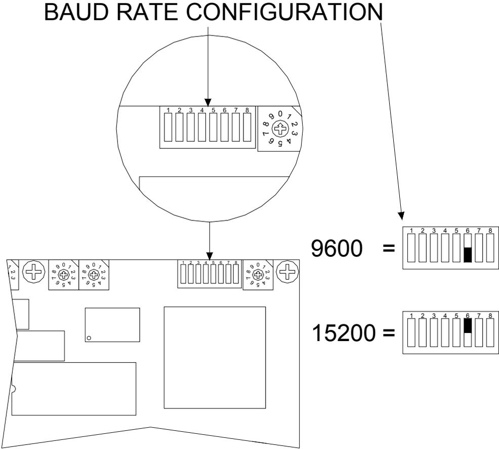
**Figure 2.11: Baud Rate Configuration**
