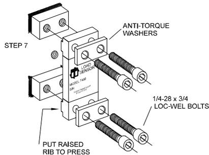
STEP 6 Remove the weld fixture. DO NOT WELD AFTER FIXTURE IS REMOVED. The 4 screws holding the pads to the fixture and the 1 center screw may be discarded. DO NOT USE THE FOUR 1 INCH LONG SCREWS TO ASSEMBLE SENSOR. The sensor kit contains four 3/4 inch long screws for assembling the sensor to the press member. Weld pad surface must be clean – no weld bumps, scratches, etc. Be sure the weld pad tapped holes are clean and bottom of holes are free of weld flash.
