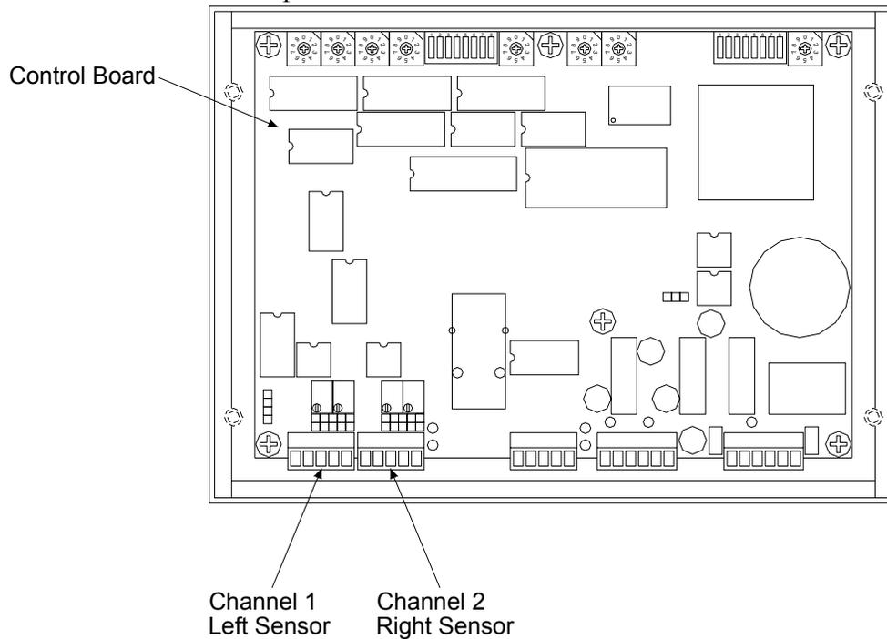
**Figure 1.8: Sensor Input Locations**
