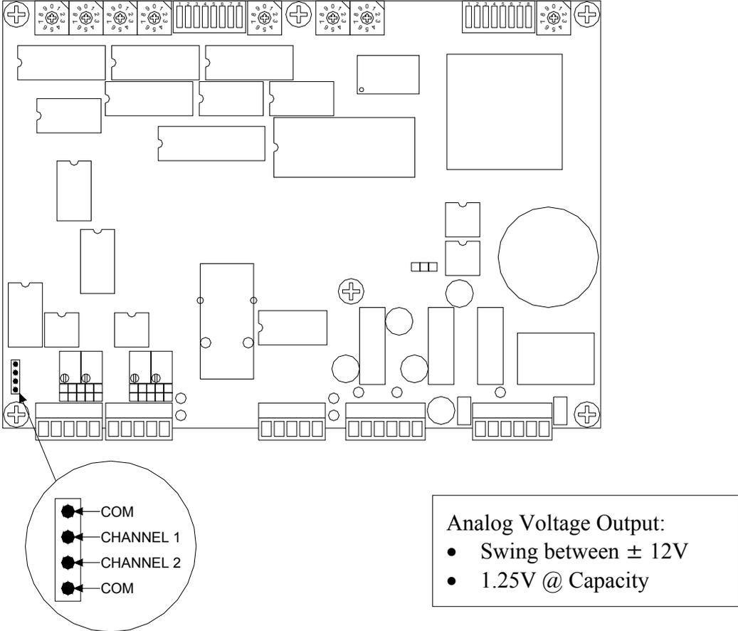
**Figure 1.11: Analog Output Wiring**
