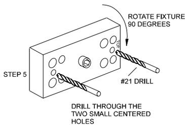
STEP 5 Loosen the fixture. Rotate the fixture 90 degrees clockwise. Tighten the center screw of the fixture. Insert the number 21 drill into the small centered hole and drill out both holes to a depth of 3/8 of an inch. These holes are for mounting the sensor enclosure. The fixture does not allow for tapping these holes. They are tapped without the fixture. Enclosure mounting is not done in metric.
