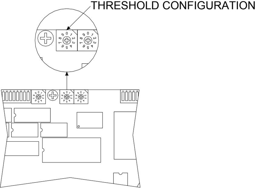
**Figure 2.4: Threshold Configuration**
