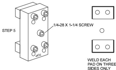
STEP 5 Weld the weld pads to the press member. (BE SURE TO ONLY WELD THE WELD PADS ON THREE SIDES AS SHOWN.) A single pass is sufficient. Do not remove the fixture until slag is removed and or assembly has cooled. When welding cast iron, use a dry nickel rod such as: Lincoln Electric "Soft Weld", Hobart "NI Cast 99", or MB Weld Prod. "MG 210. Strike arc on steel then puddle into the cast iron.
