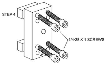
STEP 4 Remove the fixture from the press member. Bolt the weld pads to the fixture with 1/4-28 by 1 inch long socket head cap screws provided. Reattach the fixture with the weld pads bolted on using the center hole as in Step 3. Orient the fixture as shown.
