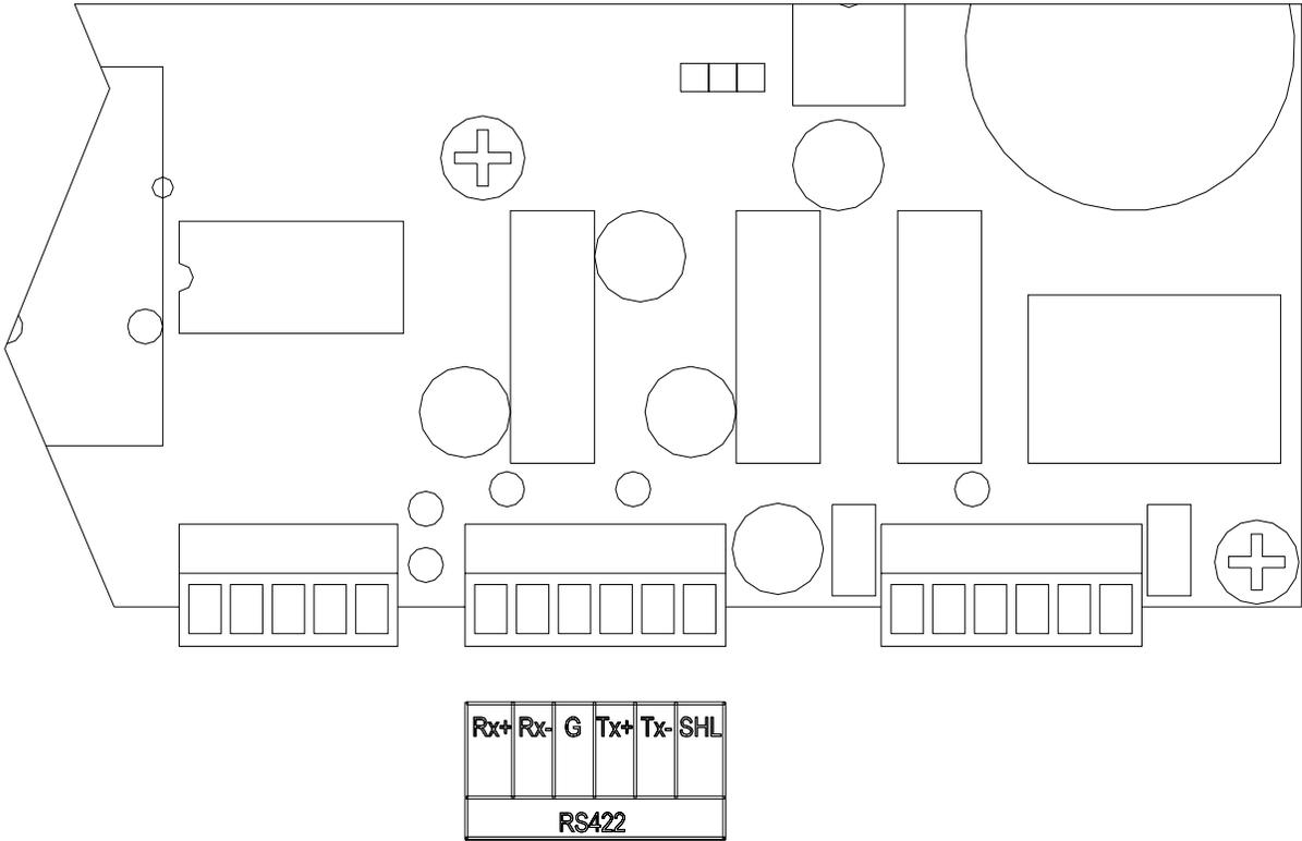
**Figure 1.15: Serial Connection**
