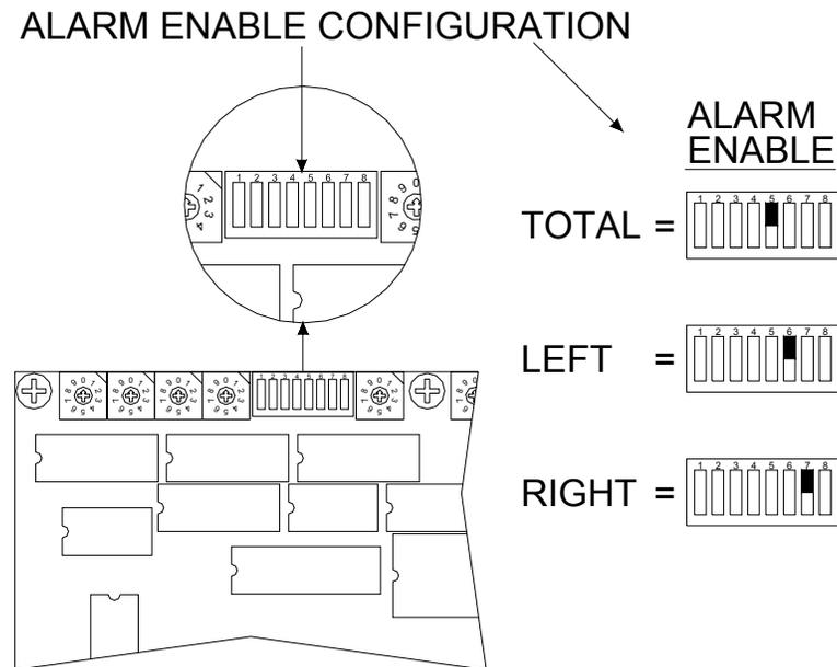
**Figure 2.6: Alarm Enable Configuration**
