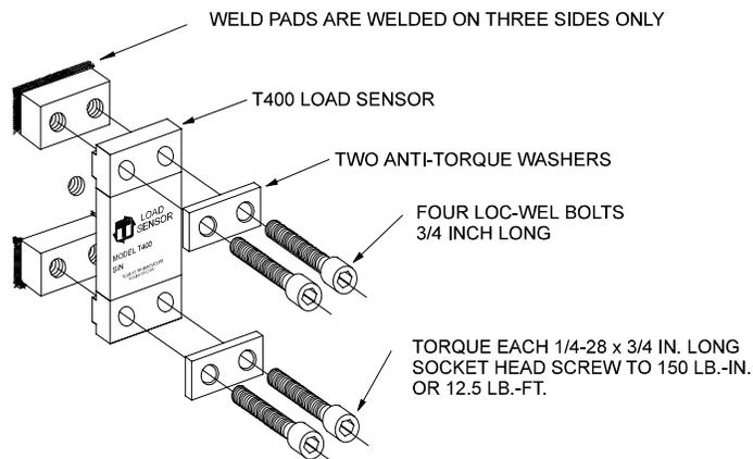
The above illustrations represent the proper arrangement of Model T400 Load Sensor kit parts using either the Drill and Tap method or the Weld method.
