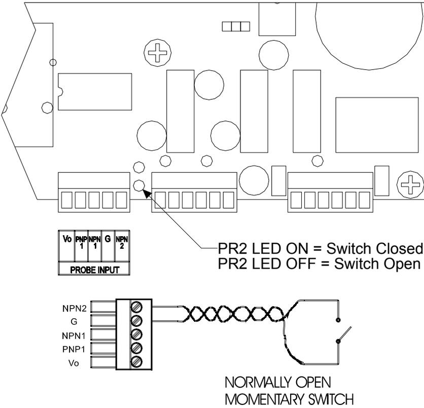
Figure 1.14: External Reset Switch Wiring
