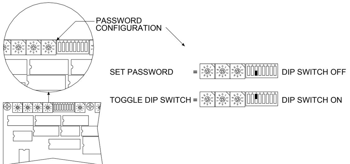
**Figure 2.7: Password Configuration**
