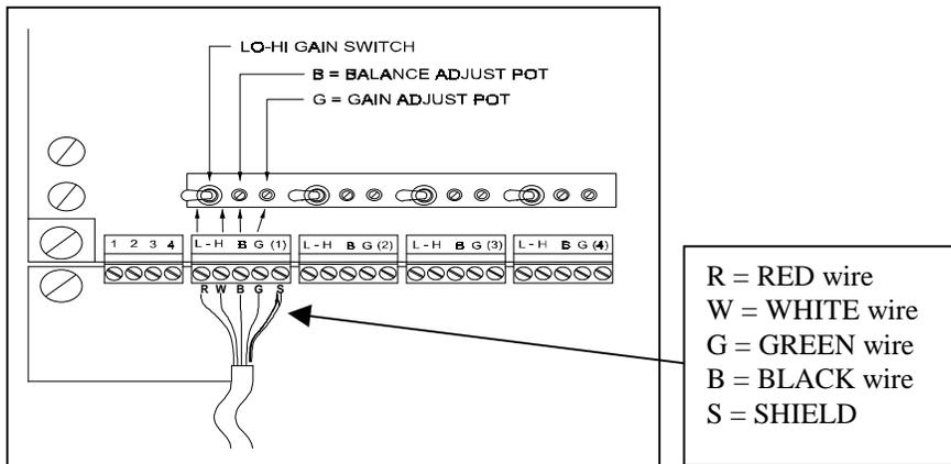
**Figure 3: Proper Cable and Shield hook-up**
